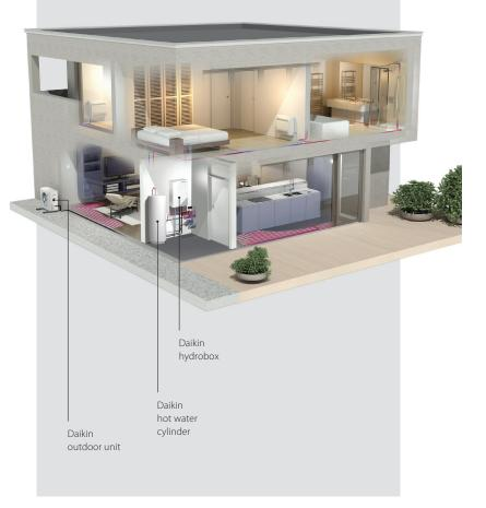
\* 4kW Daikin Altherma LT Split tested in accordance to EN 14511 at A7 W35 (COP 5.04)
